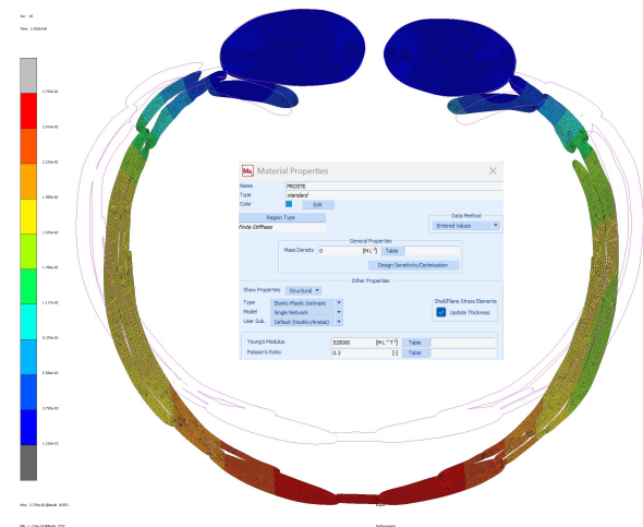
Figure 2: Displacement result for plane strain FEM model in Marc Mentat
