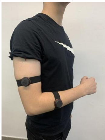
Figure 1: sensors attached to the hand with an elastic band
