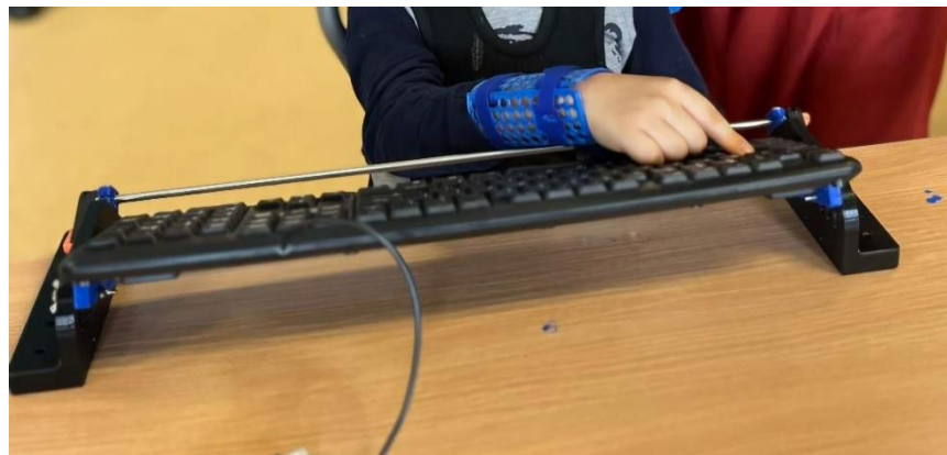
Fig. 1. Arm stabilizing keyboard overlay in use during the test in Dąbrowa Górnicza
