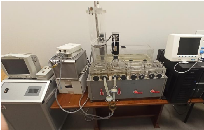
Figure 1: Hybrid cardiovascular simulation system with the POLVAD LVAD connected for the studies.
