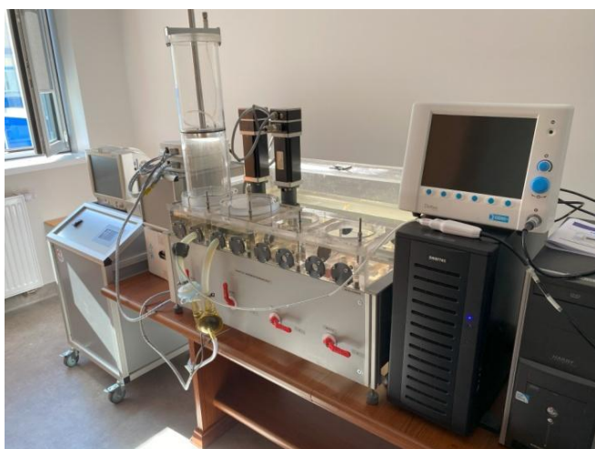
Figure 1: The mock up circulatory system used for model studies
